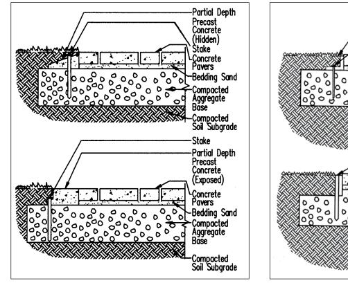
Figure 5. Partial depth precast concrete edge.
