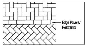
*Figure 1. Change in laying pattern direction.*
