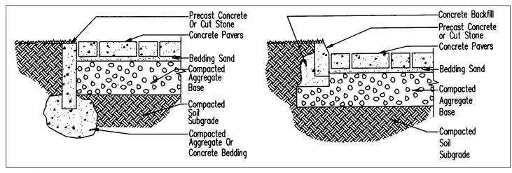
Figure 4. Precast concrete/cut stone.
