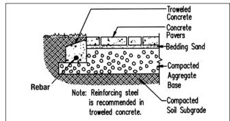
Figure 9. Troweled concrete edges.
