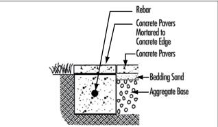
Figure 10. Submerged concrete edge.
