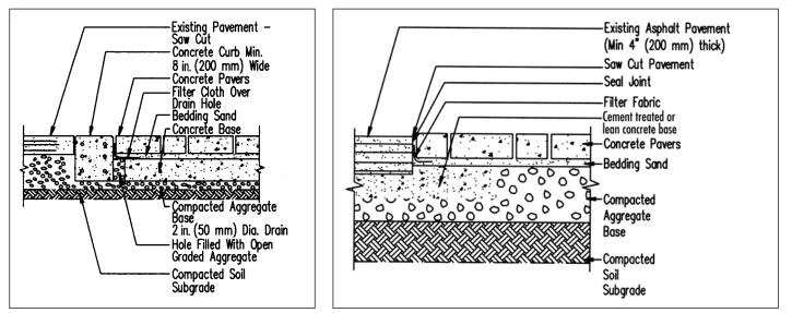
Figure 13. Crosswalk with concrete base.
