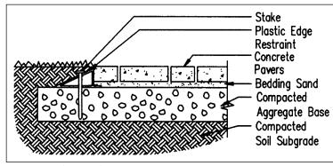
Figure 7. Plastic edge restraint.
