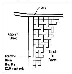
Figure 12. Concrete beam.
